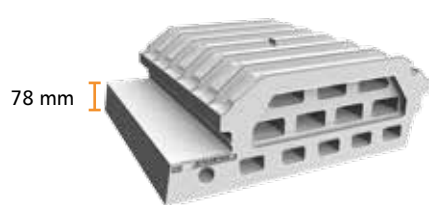
Entrevous Isoleader 27 Up = 0,27 W/m 2 .K – Rp = 3,35 m 2 .K/W
