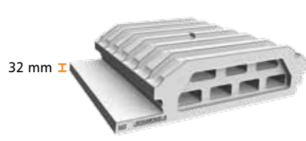
Entrevous Isoleader 39 Up = 0,39 W/m 2 .K – Rp = 2,25 m 2 .K/W
