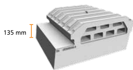
Entrevous Isoleader 18 Up = 0,18 W/m 2 .K – Rp = 5,22 m 2 .K/W
