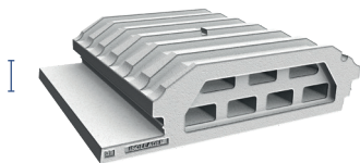
ENTREVOUS ISOLEADER 39 Up = 0,39 W/m².K - Rp = 2,25 m²K/W
