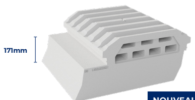
ENTREVOUS ISOLEADER 15 Up = 0,15 W/m².K - Rp = 6,30 m²K/W
